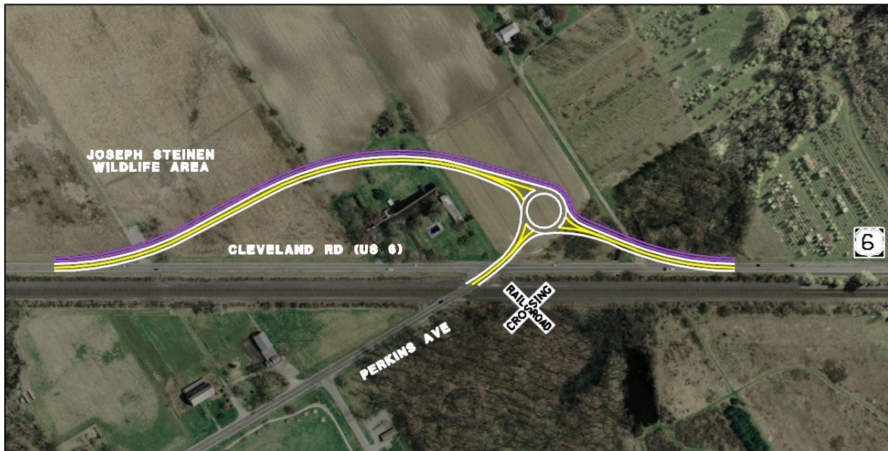
Figure 32: Alternative CI – Perkins Avenue Roundabout
